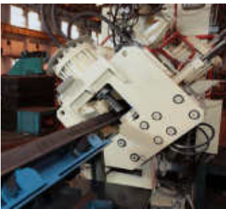
Bending - 12-metre hydraulic press brake machine from LVD (Belgium)
